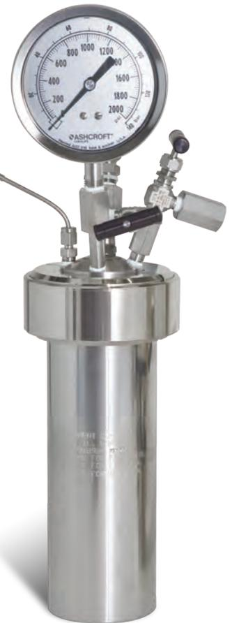
**Model 4760-600mL, with VGR, O-ring seal, and single inlet valve.**
