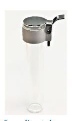
Sampling tube Sample can be protected from evaporation and falling bacteria by a protection lid
