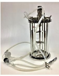
Sampling unit can be autoclaved with a vessel
