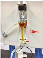
Sampling chamber Sampling chamber measures 10mL of sampling volume
